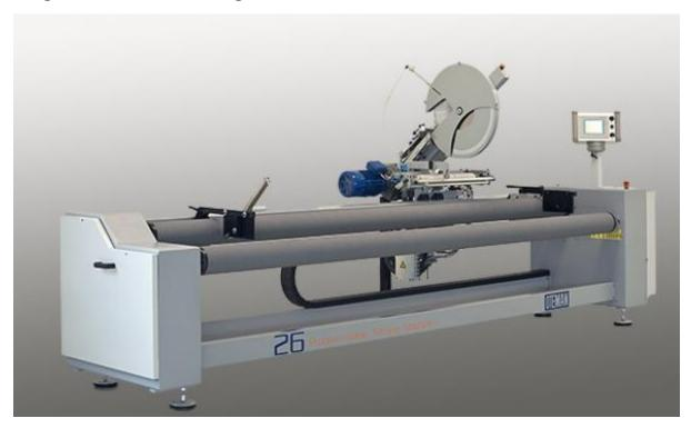
The 26P is the answer to fast and precise roll slitting. Equipped with two steel rollers to support the material, has been design to cut the most varied materials into strips, as textiles, non woven, carpets, synthetic leather, adhesives, fiber glass, PVC etc.
