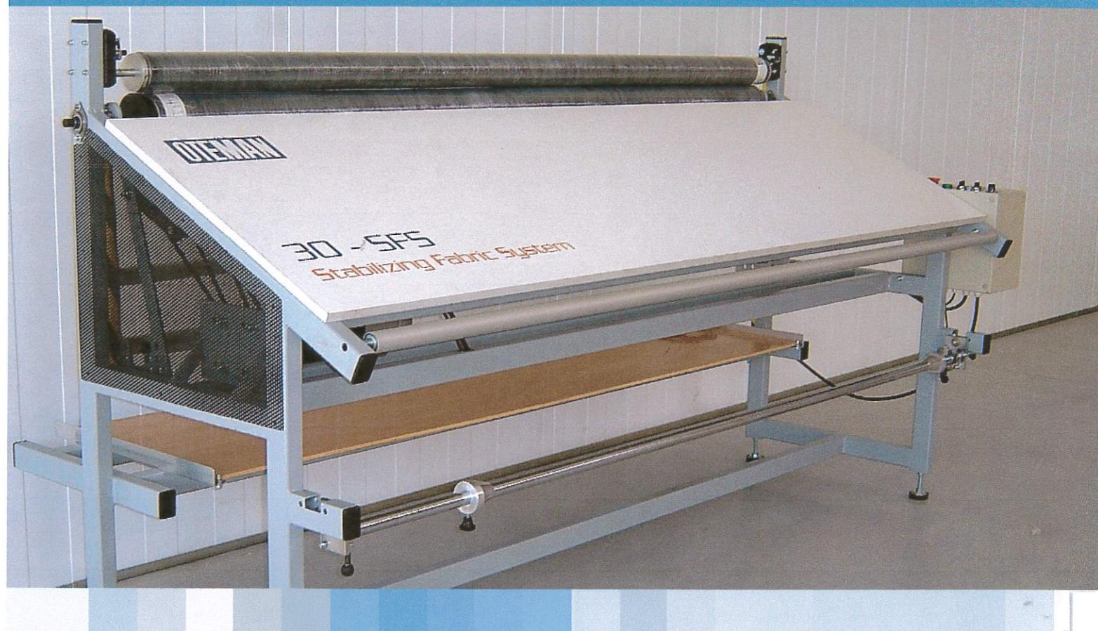
Machine to unroll the fabric and fold it into flat fold. The folder consists of two cylinders able to work in a swinging motion, making it easy to fold the fabric for later stabilizing.
