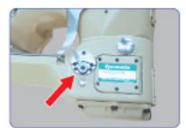
Differential Feed Amount Easily adjustable by outer lever.
